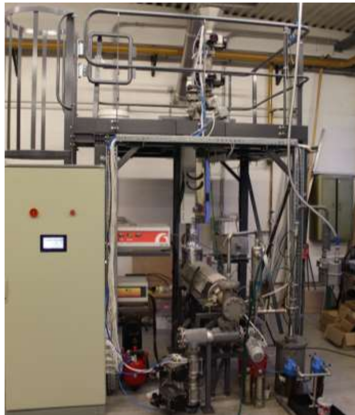
Figure 1 The experimental gasification technology
