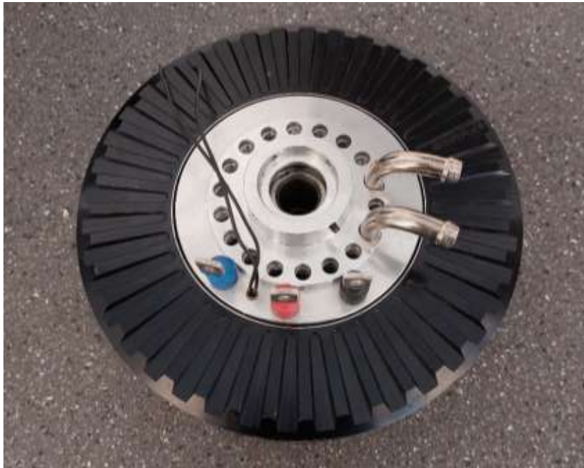
1. Figure EMRAX 228 - the electric motor powering our racecar.
