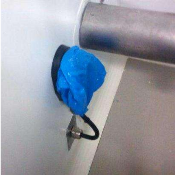
Picture 3 inhibition with plastic disposable shoe cover
